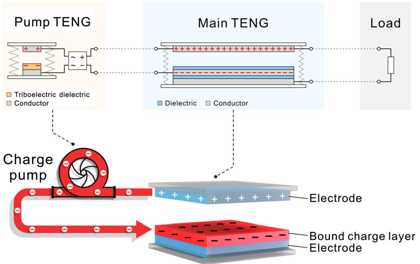
**Figure 36.** Concept of the charge-pumping TENG and the detailed structure of the device. Reprinted from [123], Copyright (2018), with permission from Elsevier.
