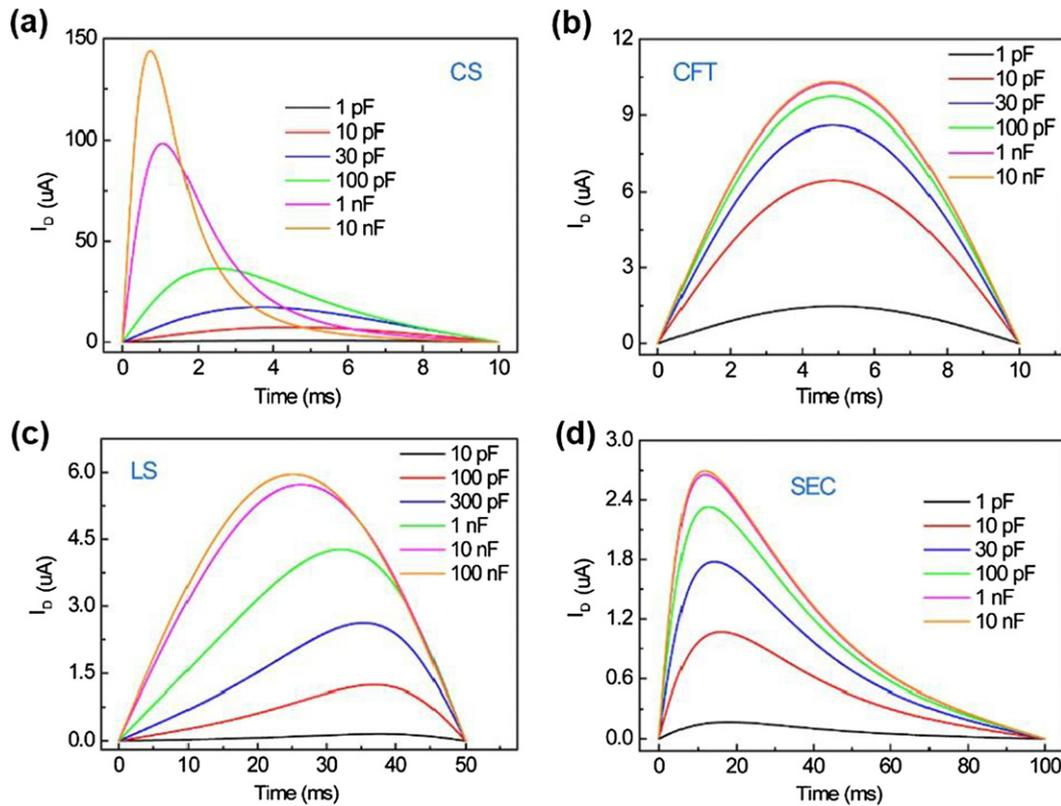
**Figure 31.** Numerical calculations of the displacement current ( $I_D$ ) in the TENG charging system.  $I_D$ -time relationships at different load CAs for (a) CS mode, (b) contact freestanding triboelectric-layer (CFT) mode, (c) lateral sliding (LS) mode and (d) single-electrode contact (SEC) mode TENGs. Note that one side edge effect of the TENGs has been considered when calculating the  $I_D$ . Reprinted from [104], Copyright (2019), with permission from Elsevier.
