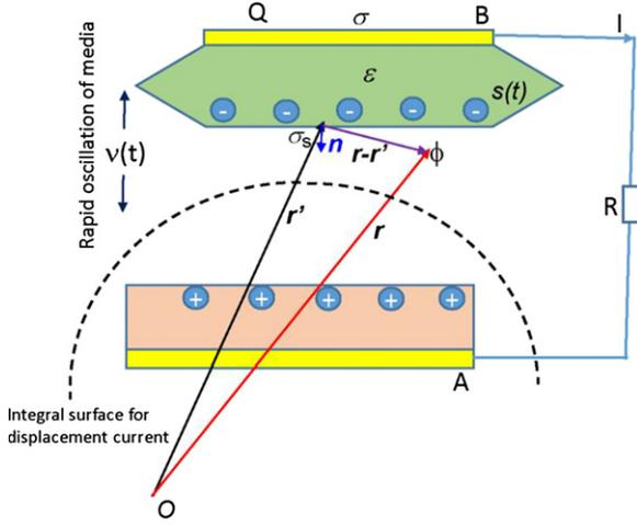
**Figure 25.** Schematic illustration of a general TENG and the associated coordination system for theoretical study.
