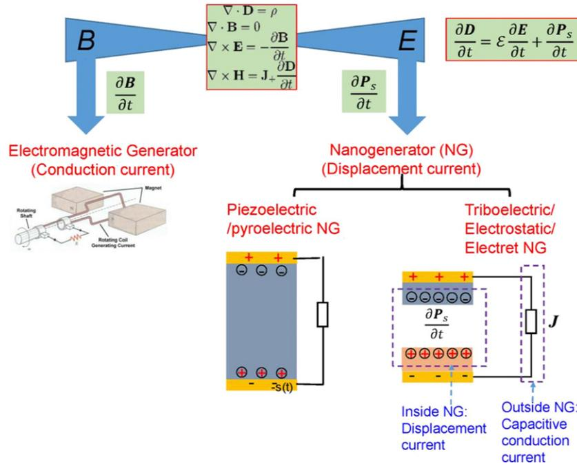
**Figure 26.** Schematic showing the conduction current-dominated EM generator and displacement current-dominated NGs based on piezoelectric/pyroelectric, triboelectric/electrostatic/electret effects. The difference and relationship between the two are illustrated.
