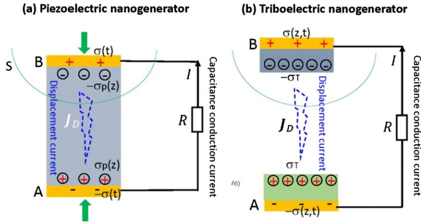
Figure 27. (a) Thin film-based PENGs and (b) CS mode TENGs.
