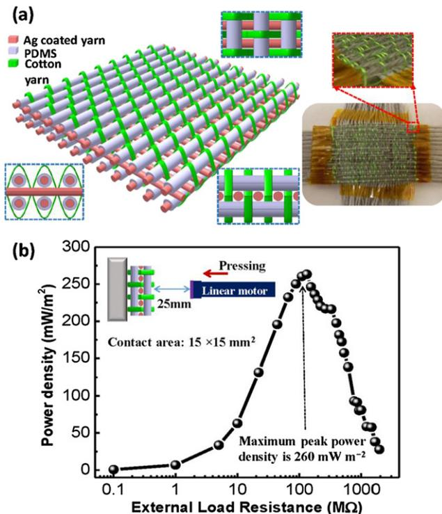
**Figure 42.** Fiber/textile-based TENG. (a) Schematic illustration and photograph of the 3D orthogonal woven TENG (3DOW-TENG). (b) Measuring conditions and maximum peak power density of the 3DOW-TENG. [148] John Wiley & Sons. © 2020 WILEY-VCH Verlag GmbH & Co. KGaA, Weinheim.
