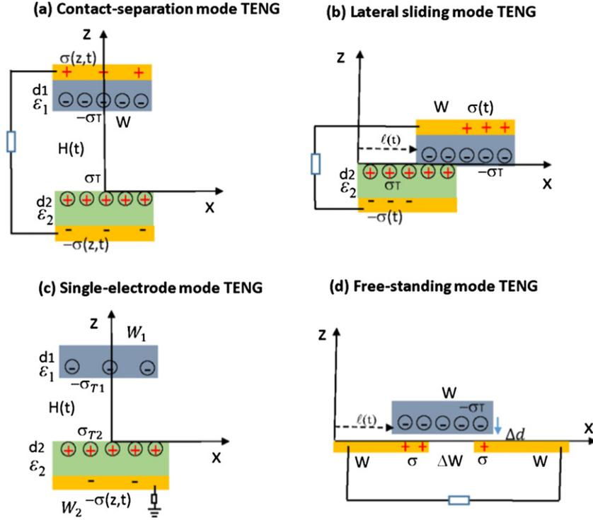
**Figure 28.** Coordination system and mathematical parameters defined for describing (a) CS, (b) lateral-sliding mode, (c) single-electrode mode and (d) free-standing mode TENGs, respectively.
