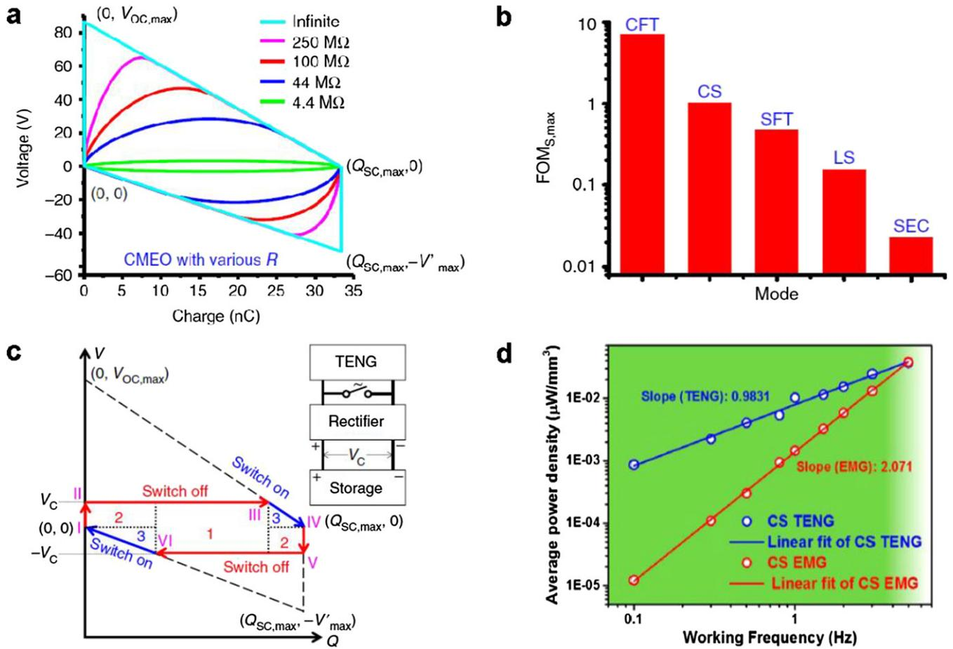
**Figure 33.** FOMs, effective energy storage, and ‘killer applications’ of the TENG. (a) Cycles of the maximized energy output (CMEO). (b) The structural FOM for various modes of TENGs. (c) The effective energy storage strategy for TENG. Reproduced from [112]. CC BY 4.0. (d) The high output of TENG compared with EM generator, demonstrating low-frequency energy harvesting as a ‘killer application’ of TENGs. [113] John Wiley & Sons. © 2016 WILEY-VCH Verlag GmbH & Co. KGaA, Weinheim.
