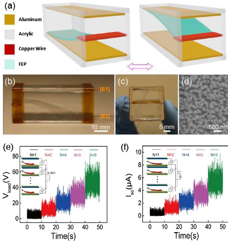
**Figure 44.** Harvesting energy from wind by TENG. (a) Schematic diagram of the TENG. (b) and (c) Photographs of the TENG. Reprinted with permission from [172]. Copyright (2013) American Chemical Society. (d) SEM image of the etched FEP film surface. (e) and (f) Rectified OC voltage and SC current of several units in serial and parallel connection, respectively. Reprinted from [171], Copyright (2020), with permission from Elsevier.
