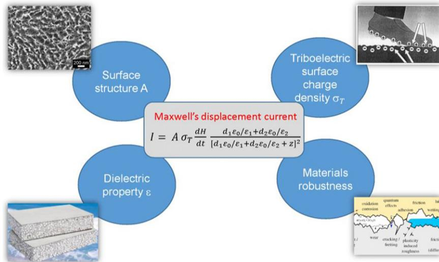
**Figure 35.** Using the theoretical result of displacement for CS mode TENG, we show here the requirements and research directions for materials in order to maximize the output of the TENG.
