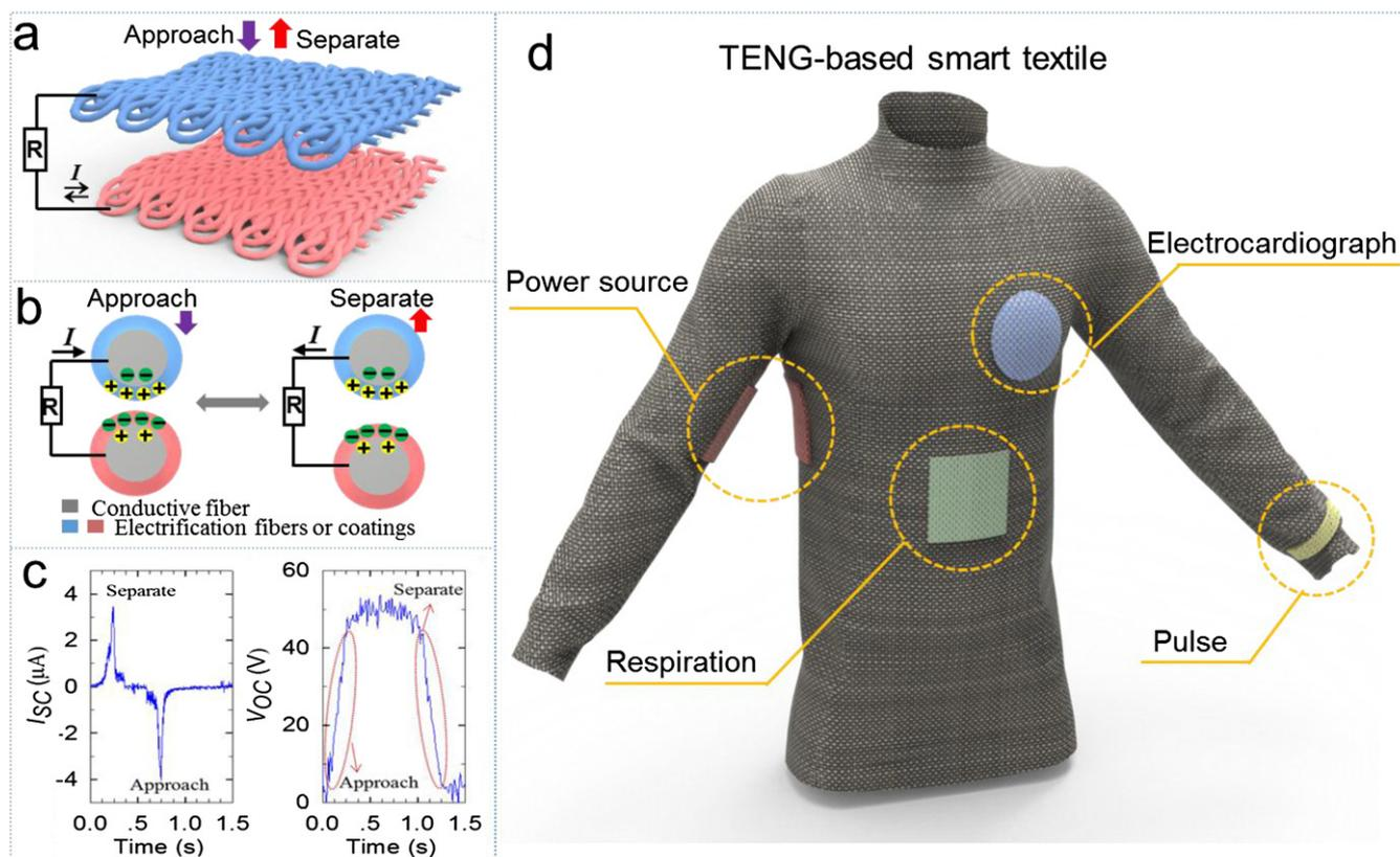
**Figure 41.** TENG-based smart textiles. (a) A scheme of a CS mode TENG textile, (b) the mechanism of how a fiber-based TENG works in response to the relative motion of fibers, and (c) corresponding typical output SC current and OC voltage. (d) The potential applications of TENG-based smart textiles. [154] John Wiley & Sons. © 2015 WILEY-VCH Verlag GmbH & Co. KGaA, Weinheim.
