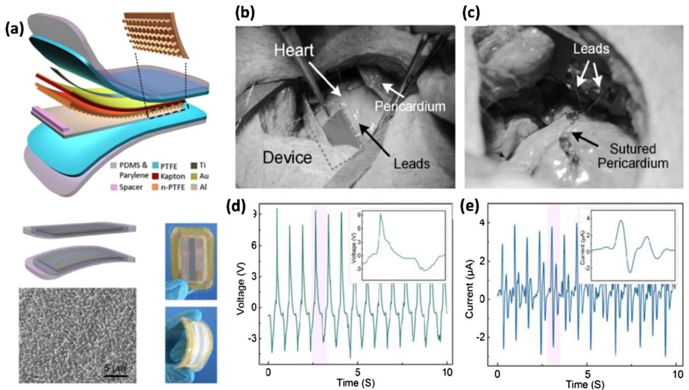
**Figure 39.** Pacemakers driven by implanted TENGs. (a) The structure and fabrication of the TENG. (b) and (c) The *in vivo* implantation process of the TENG in animal experiments. Reproduced from [143]. CC BY 4.0. (d) and (e) The output voltage and current of the TENG in responding to the cardiac motion. (a), (d) and (e) Reprinted with permission from [141]. Copyright (2016) American Chemical Society [143]
