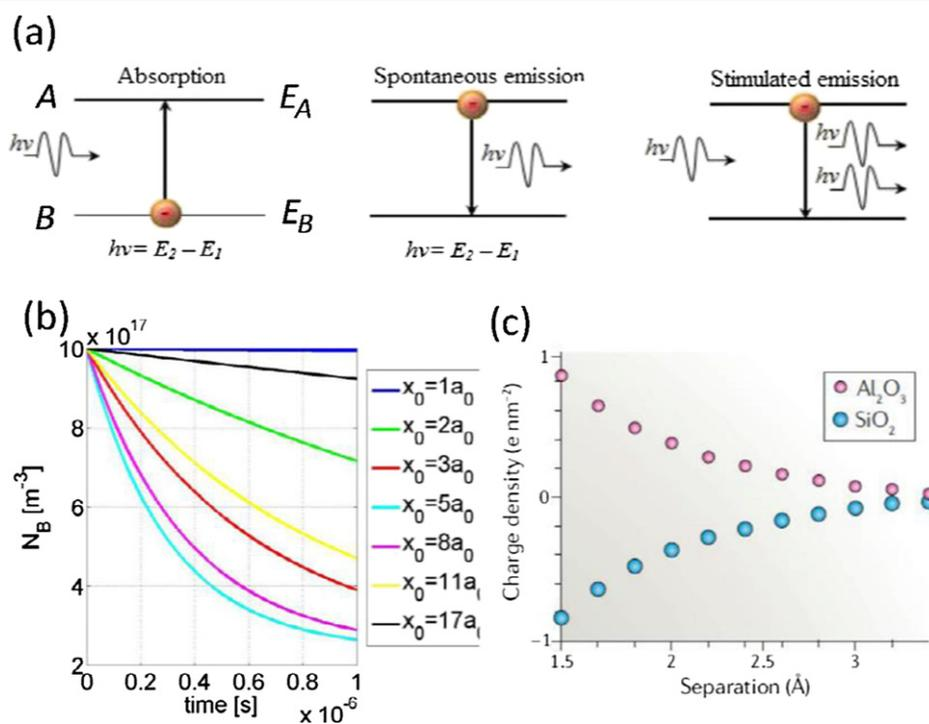
**Figure 11.** (a) Absorption, stimulated emission and stimulated absorption in atomic systems. (b) Electron dynamics and CE in a system of two atomic systems A and B.  $a_0$  is the Bohr radius: 0.053 nm. Reproduced from [58]. CC BY 4.0. (c) Charge transfer between  $\text{Al}_2\text{O}_3$  and  $\text{SiO}_2$  surfaces as a function of their separation calculated using DFT. Reprinted from [60], Copyright (2016), with permission from Elsevier.
