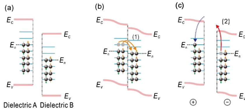
**Figure 9.** Charge transfer (a) before contact, (b) in contact, and (c) after contact between two different insulator dielectrics for a case where  $E_n$  of the former is higher than that of the latter and the band structure model holds.
